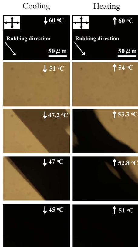
FIG. 2. (Color online) POM images of LC textures showing anchoring transitions in the cooling (left) and heating (right) processes.
