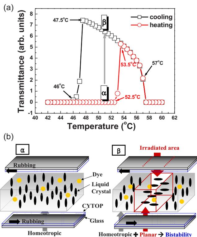
FIG. 1. (Color online) (a) Transmittance intensities of an orientated sample of CCN-47 doped with C153 (0.5 wt %) under crossed polarizers as a function of temperature. (b) Schematic illustration of light-induced anchoring transition and bistability.
