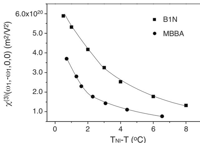
FIG. 4. Variation of nonlinear static susceptibility  $[\chi^{(3)}(\omega_1, -\omega_1, 0, 0)]$  as a function of temperature. Data corresponding to the solid squares are obtained from the present bent-core compound and those of solid circles are from Ref. [18]. Solid lines are drawn as guides to the eye.
