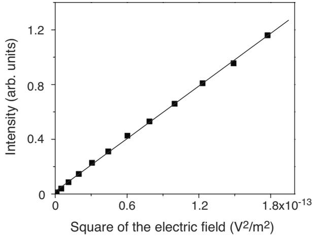
FIG. 1. Transmitted intensity of the modulated signal ( $I_{ac}$ ) as a function of square of the applied field measured at a frequency 2 kHz. The solid line is the best fit obtained from a least-squares method. The sample used is also shown at the top of the figure.
