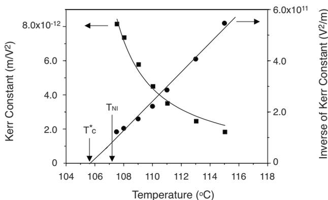
FIG. 3. Solid squares represent the variation of Kerr constant ( $B$ ) as a function of temperatures. The inverse Kerr constant  $1/B$  is also plotted by solid circles to show the Landau–de Gennes-type temperature dependence. Actually  $1/B \propto (T - T_C^*)$  is shown by the best fit to the data points from a least-mean-squares method.  $T_C^*$  is found to be almost 1.5 °C below  $T_{NI}$ .
