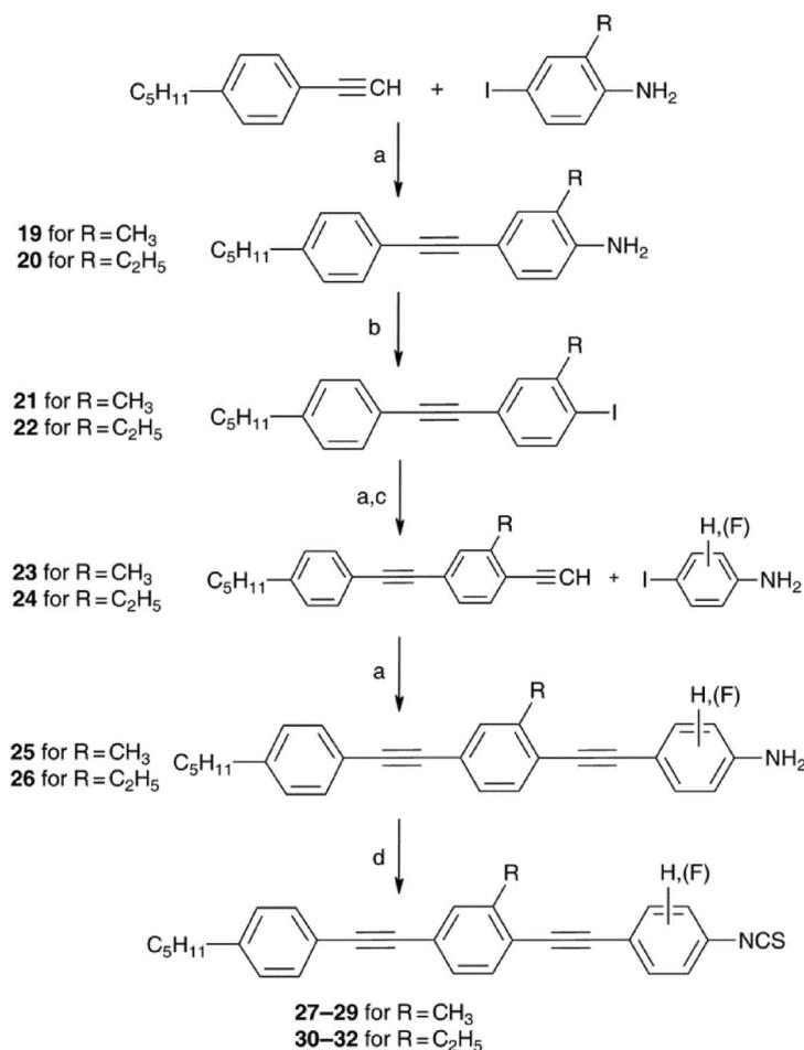
Scheme 2. Synthetic route to phenylethynyltolane liquid crystals (series 2). Synthetic conditions: a – PdCl<sub>2</sub>(PPh<sub>3</sub>)<sub>2</sub>, CuI, TEA, DBU, THF; b – HCl, dioxane, NaNO<sub>2</sub>, KI; c – NaH, toluene; d – CSCl<sub>2</sub>, CaCO<sub>3</sub>, H<sub>2</sub>O, CHCl<sub>3</sub>.
