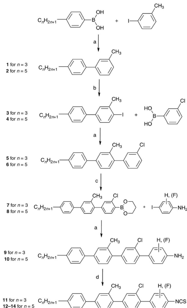
Scheme 1. Synthetic route to quaterphenyl liquid crystals (series 1). Synthetic conditions: a – Pd(OAc)<sub>2</sub>, K<sub>2</sub>CO<sub>3</sub>, Acetone, H<sub>2</sub>O; b – I<sub>2</sub>, HIO<sub>3</sub>, H<sub>2</sub>SO<sub>4</sub>, CH<sub>3</sub>COOH, H<sub>2</sub>O; c – (1) sec-BuLi, THF, –75°C, (2) B(OC<sub>3</sub>H<sub>7</sub>)<sub>3</sub>, –75°C, (3) H<sub>3</sub>O<sup>+</sup>, H<sub>2</sub>O; d – CSeCl<sub>2</sub>, CHCl<sub>3</sub>, H<sub>2</sub>O.
