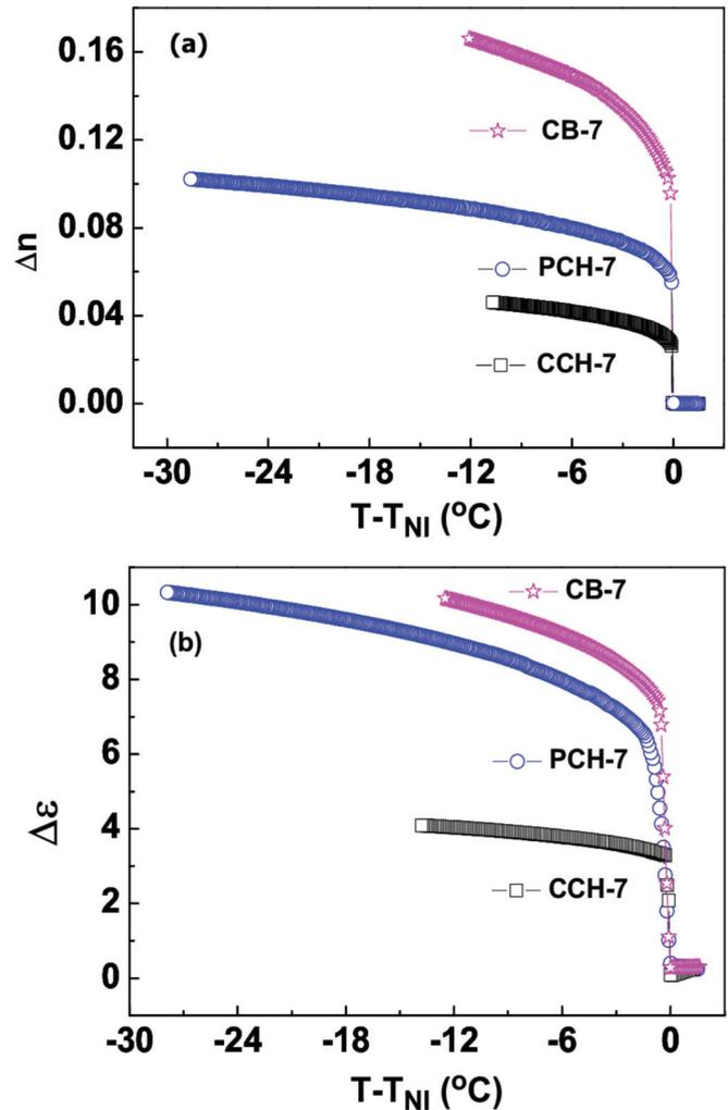
FIG. 3. (Color online) Variation of (a) birefringence  $\Delta n$  and (b) dielectric anisotropy  $\Delta\epsilon$  with shifted temperature of CB-7 (open stars), PCH-7 (open circles), and CCH-7 (open squares) liquid crystals. The dielectric constants are measured at a frequency of 4.11 kHz. Cell thickness is 5  $\mu\text{m}$ .
