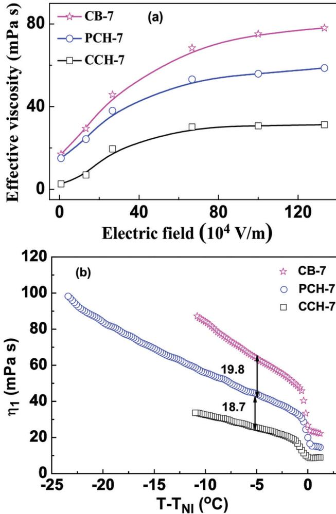
FIG. 6. (Color online) (a) Variation of effective viscosity  $\eta_{\text{eff}}$  at a fixed shear rate,  $\dot{\gamma} = 50 \text{ s}^{-1}$ , as a function of applied field at a frequency of 3.11 kHz. At high field (beyond about  $80 \times 10^4 \text{ V/m}$ )  $\eta_{\text{eff}} = \eta_1$ . (b) Variation of  $\eta_1$  as a function of shifted temperature and a fixed electric field of  $133 \times 10^4 \text{ V/m}$  ( $\dot{\gamma} = 50 \text{ s}^{-1}$ ).
