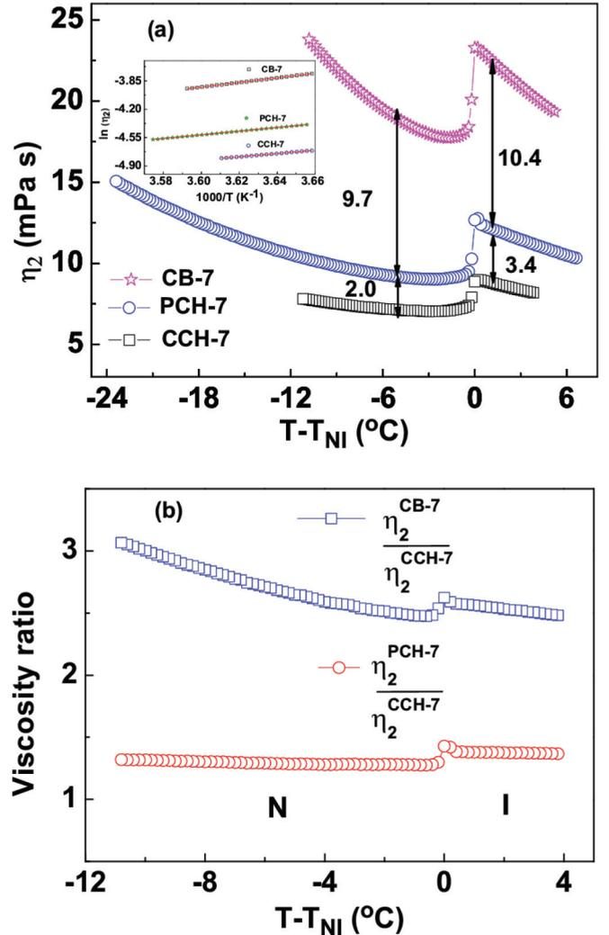
FIG. 5. (Color online) (a) Variation of  $\eta_2$  as a function of shifted temperature at a fixed shear rate,  $\dot{\gamma} = 50$  s $^{-1}$ . The inset shows the variation of the logarithm of  $\eta_2$  with the inverse of temperature in the isotropic phase. The solid lines are the best fit to the Arrhenius equation. (b) Comparison (ratio) of  $\eta_2$  of CB-7 and PCH-7 with respect to that of CCH-7.
