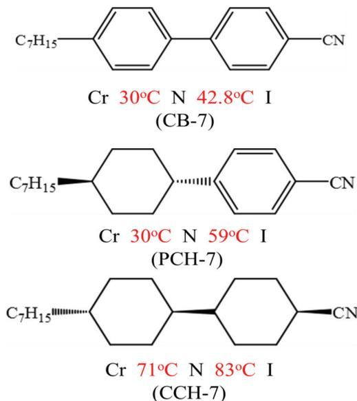
FIG. 2. (Color online) Chemical structures of CB-7, PCH-7, and CCH-7 liquid crystals and their phase transition temperatures.
